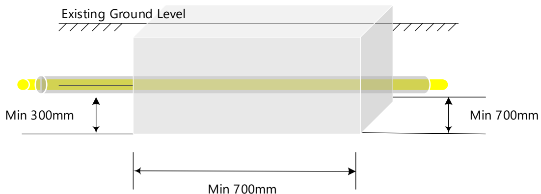
Figure 2 Galvanised Steel Inlet Service Minimum excavation requirement
