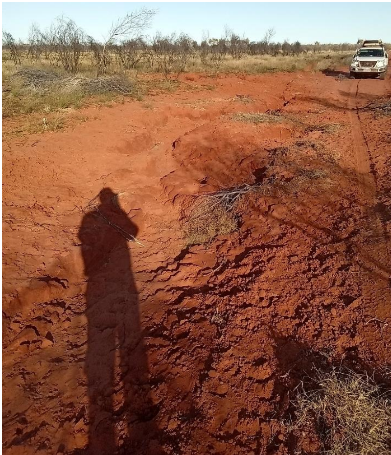
Photo 4-6. Gully erosion scored as moderate, Level 3.
