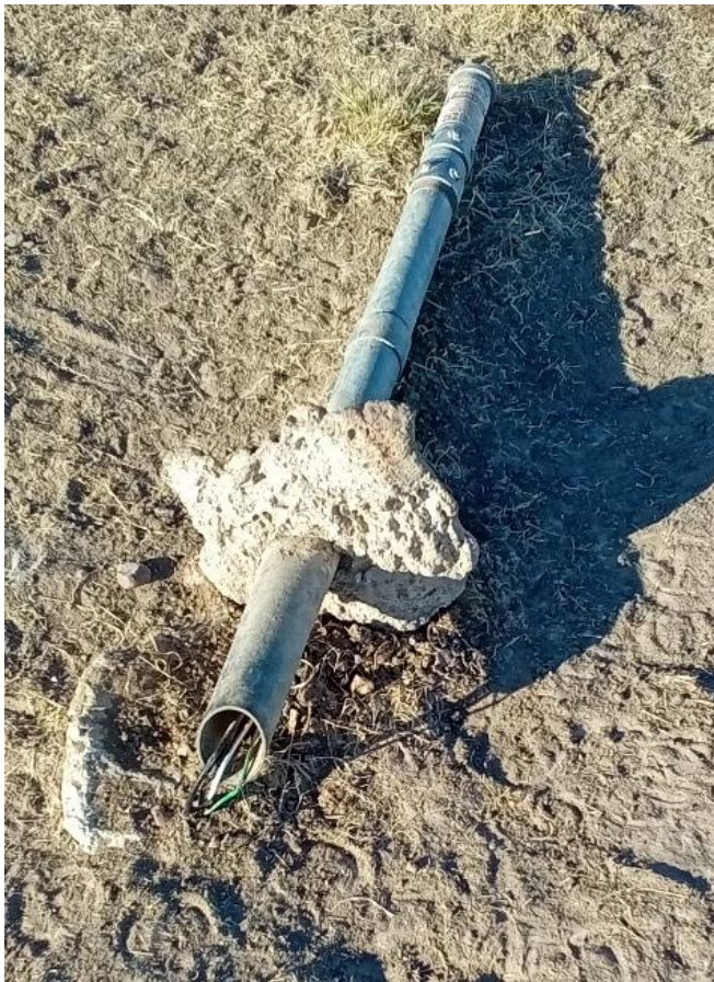
Photo 4-20. Fallen monitoring pole with exposed wires.
