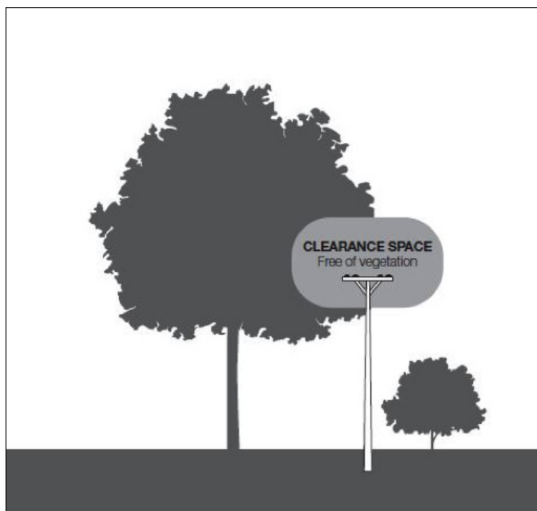
FIGURE 4 — UNINSULATED LOW VOLTAGE ELECTRIC LINE IN A LOW BUSHFIRE RISK AREA
