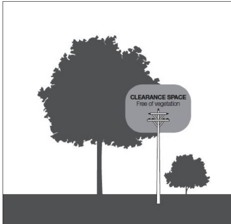
FIGURE 3 — INSULATED ELECTRIC LINES IN ALL AREAS AND UNINSULATED HIGH VOLTAGE ELECTRIC LINES (OTHER THAN 66,000 VOLT ELECTRIC LINES) IN LOW BUSHFIRE RISK AREAS
